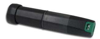
This standalone data logger can record events (detecting an input and storing the time and date), record state changes (similar to an 'event' but also recording when the input reverts back to normal) and count events (count the number of events that happen during a timed interval). Up to 32,510 events or state changes can be recorded and up to 32,510 timed intervals in event counter mode (with 65,536 events in each interval).
