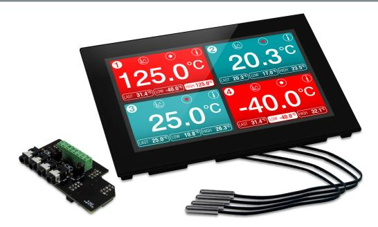
EL-SGD 70-ATP is a four-channel temperature data logger with real-time readings, trend graphing and data analysis tools.
