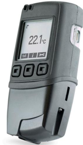
This standalone data logger measures and stores more than 250,000 temperature readings from a K, J or T-type thermocouple at a resolution of 0.1°C (0.2°F). It comes supplied with a K-type thermocouple capable of measuring from 0 to 200°C (32 to 392°F).
