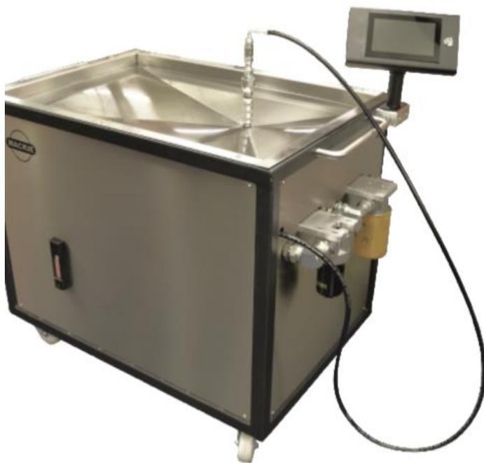
The company's first test machine was fitted with physical buttons and analogue gauges to show these values but realising technicians needed a faster and easier interface, the machine was recently re-designed using the 7 inch, capacitive, touchscreen display – the SGD 70-A.
